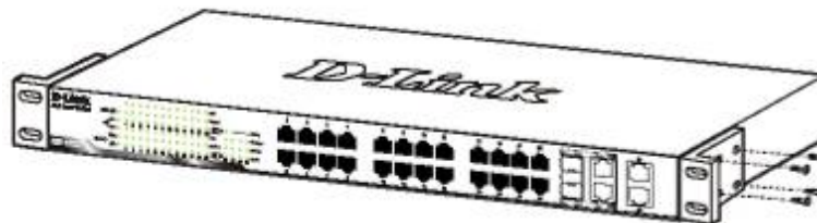
Figure 8 – Attach the mounting brackets to the Switch
